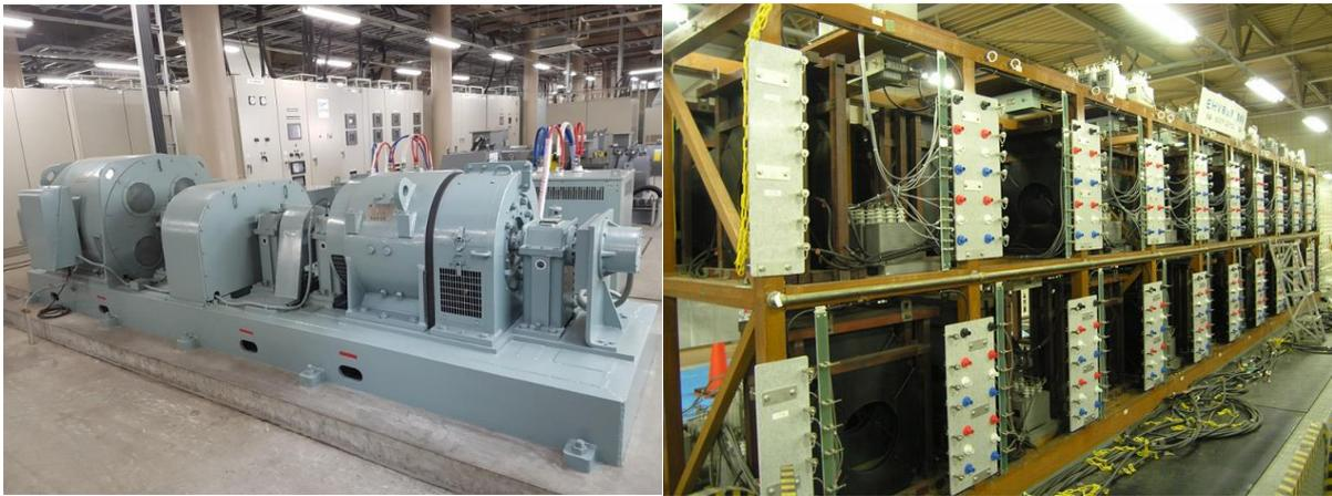
(a) Synchronous generator units (100 kVA) (b) 275 kV emulated transmission line (LL voltage: 3.3 kV)
