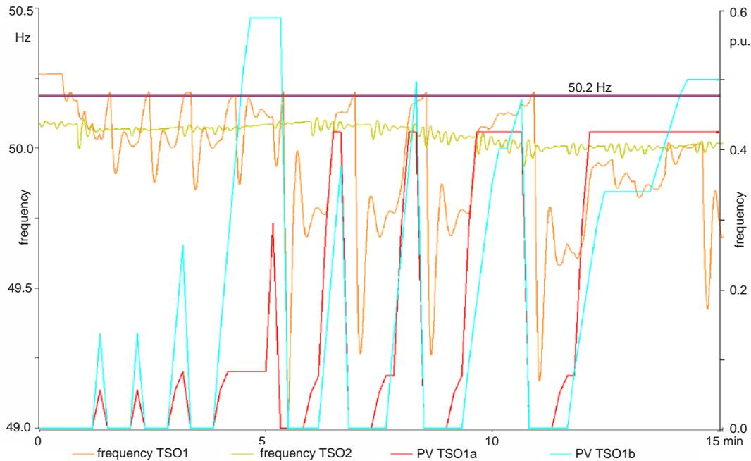
**Figure 3.9 Simulation of 50.2 Hz effect, tripping and automatic reconnection of PV in Europe [46].**
